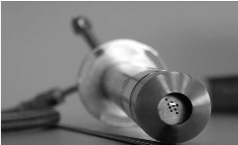
Figure 2. Multichannel fiber-optic measuring probe.
