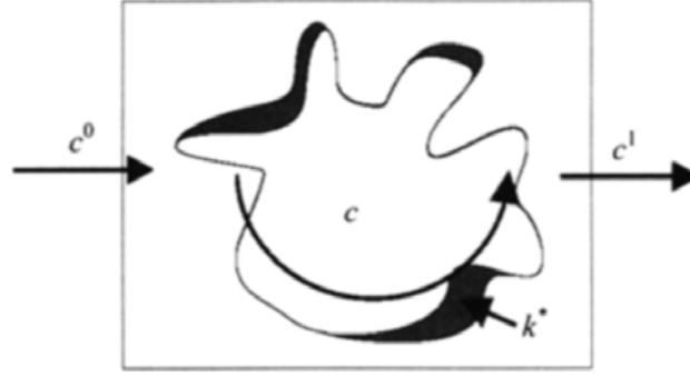
Figure 2. Conceptual diagram of PaSR reactor (the reaction zone is painted) [16].
