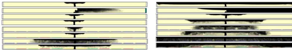
Figure 2. Smoke profiles at 50 and 170 s after the beginning of the fire for the investigated ventilation configurations (as reported, from top to down, in Table 2).
